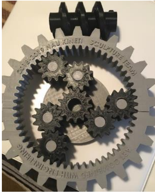
Figure 3.1: Planetary Gear System
