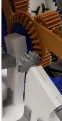
Figure 5.1: Bevel gear on Carrier
